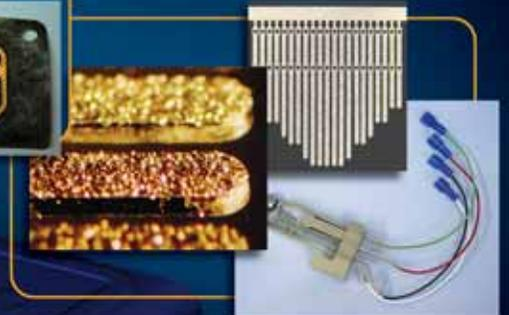
PI technology begins with 15 micron metal coated diamond particles. These diamond particles are selectively electroplated onto the substrate area using a modified PCB process. PI creates a "micro bed-of-nails" with 50,000 contact points per square inch. It makes a gas-tight electrical contact by penetrating the oxide layer, rather than the traditional wiping action of standard contactors. PI produces contact resistance below 3 milliohms.
