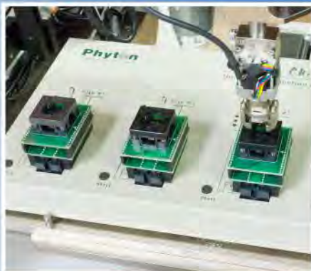
Pickup Head Closes Programmer Sockets
